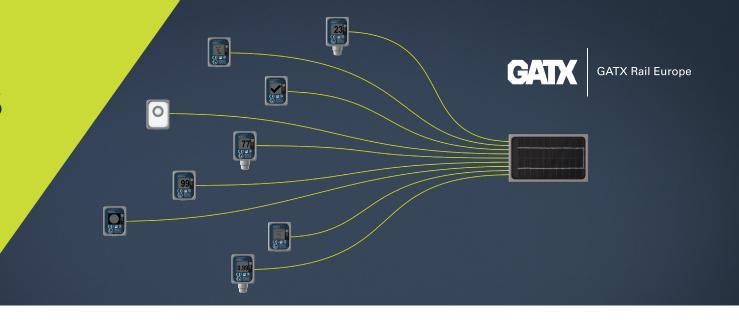
The temperature sensor can be used to monitor product quality, heating devices and valve temperature. Additionally it can be used for temperature drop/spike alerts. It can also be integrated with your existing logistics applications.
