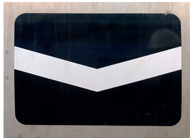
Fig 2.6: Label: Residual quantity drainage
