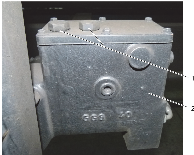
Figure 6.1: Emergency actuation bolts on the hydraulic pump
