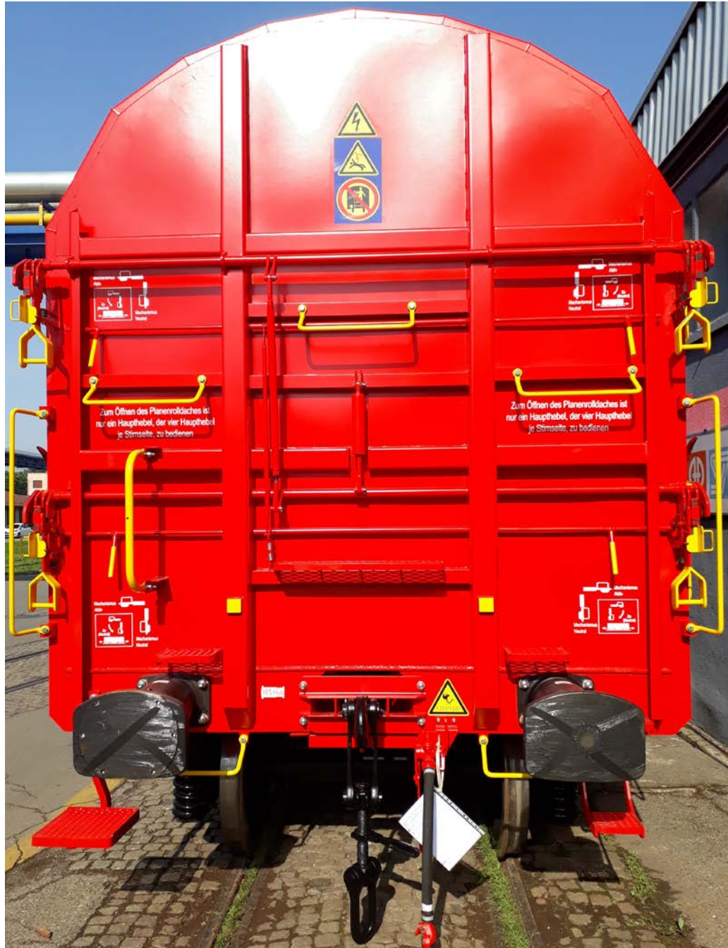
Figure 18 Steps for crossing the wagon
